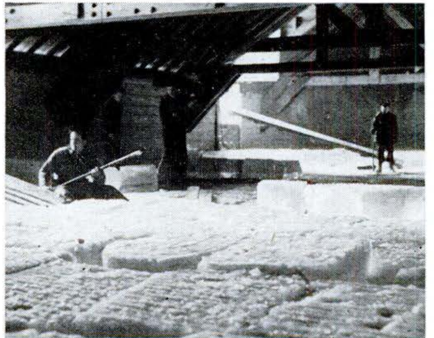
9. At 10 miles an hour , the cakes slither down a chute to the packing crews. Keyman is the switcher, who must catch the quarter-ton blocks and guide them to where packers are working.
